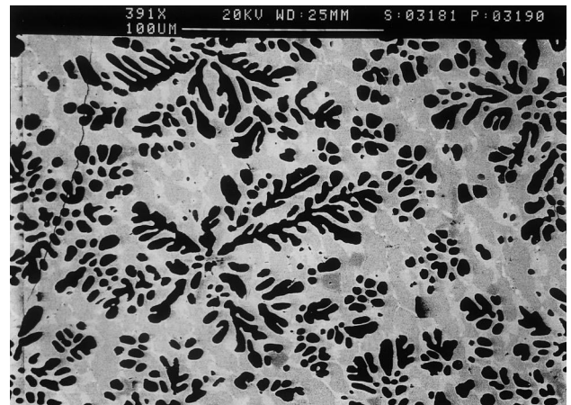
Fig. 4. Alloy N. 9: dendritic formation of Yb 5 Sn 3 (black), Ag 2 Yb 3 (grey) and Ag 3 Yb 5 (light grey).
